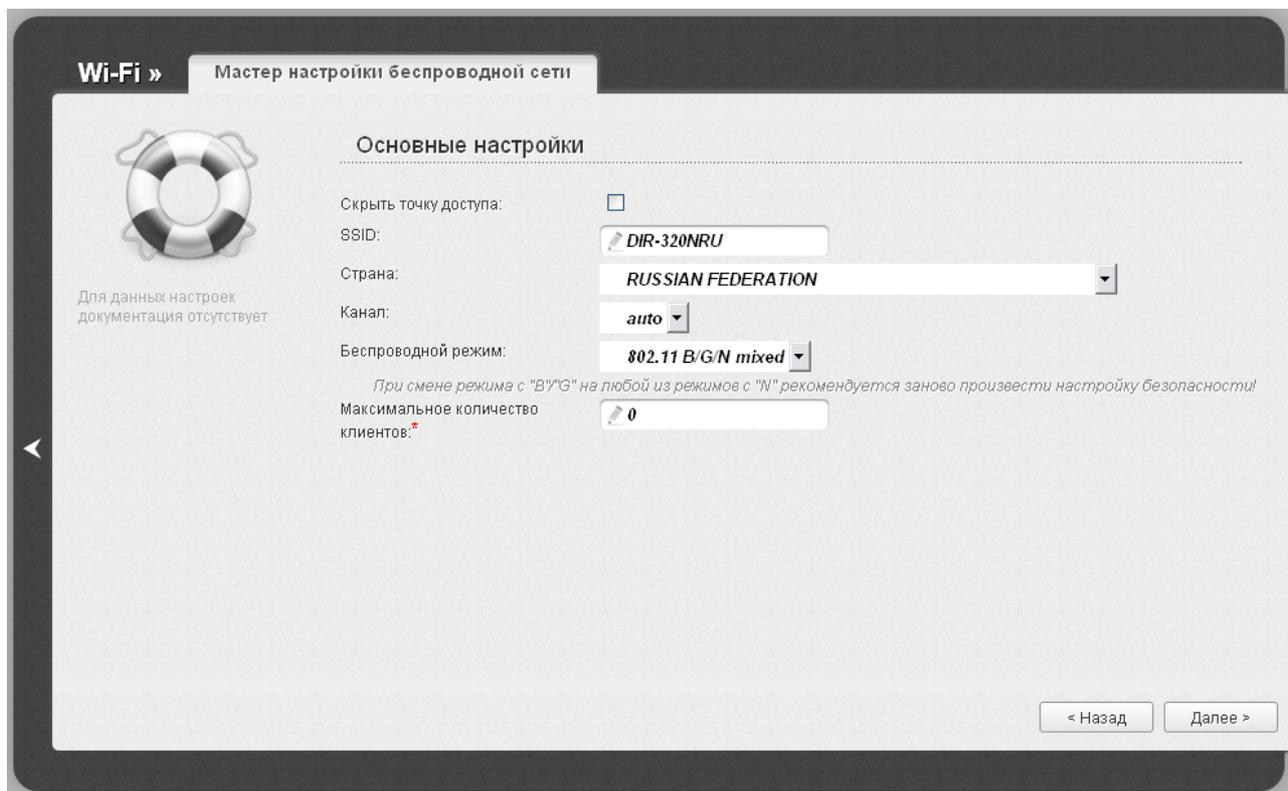
The screenshot shows the 'Wi-Fi' configuration page, specifically the 'Master settings for wireless network' (Мастер настройки беспроводной сети) section. The 'Basic settings' (Основные настройки) are displayed. On the left, there is a lifebuoy icon and a note: 'For these settings, documentation is missing' (Для данных настроек документация отсутствует). The settings are as follows:
