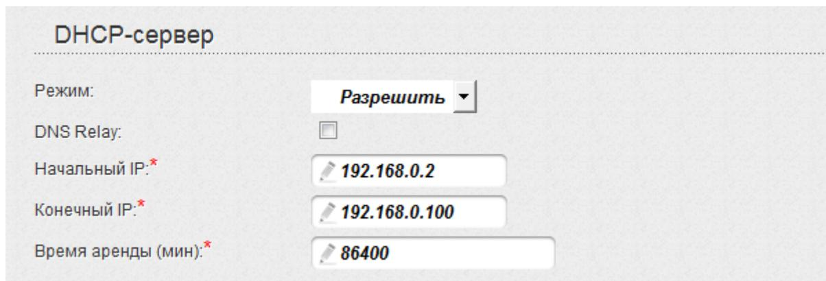
The screenshot shows the DHCP server configuration page. It has a title 'DHCP-сервер' and a dotted line separator. Below are five settings: 'Режим:' with a dropdown menu set to 'Разрешить'; 'DNS Relay:' with an unchecked checkbox; 'Начальный IP:\*' with the value '192.168.0.2'; 'Конечный IP:\*' with the value '192.168.0.100'; and 'Время аренды (мин):\*' with the value '86400'. Each value field has an edit icon.
