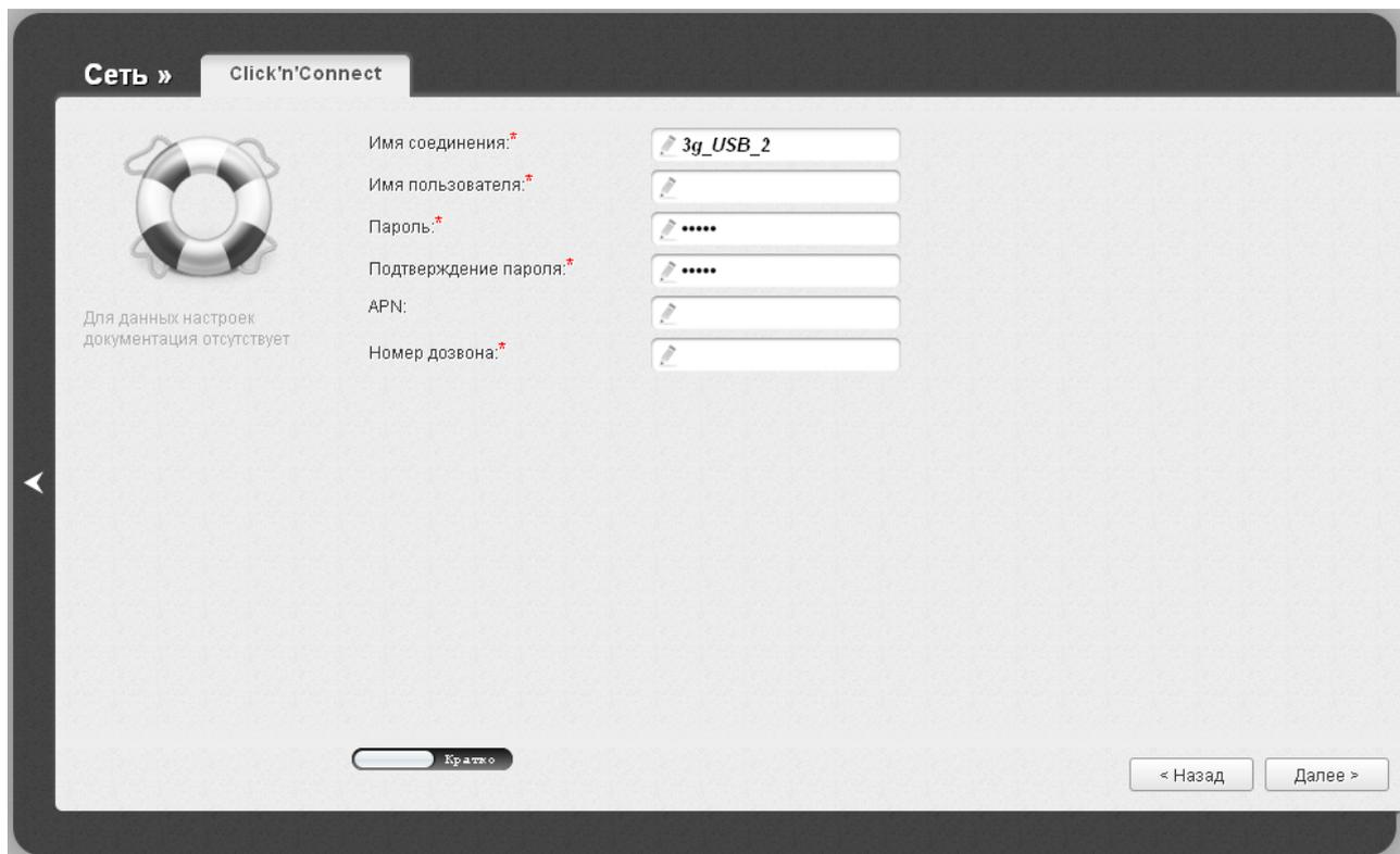
The screenshot shows the 'Сеть » Click'n'Connect' configuration page for a 3G connection. On the left, there is a lifebuoy icon and a note: 'Для данных настроек документация отсутствует'. The main area contains several input fields with red asterisks indicating required fields:
