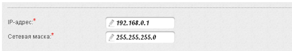
The screenshot shows the LAN configuration interface. It features two input fields: 'IP-адрес:\*' with the value '192.168.0.1' and 'Сетевая маска:\*' with the value '255.255.255.0'. Each field has a small edit icon to its left.
